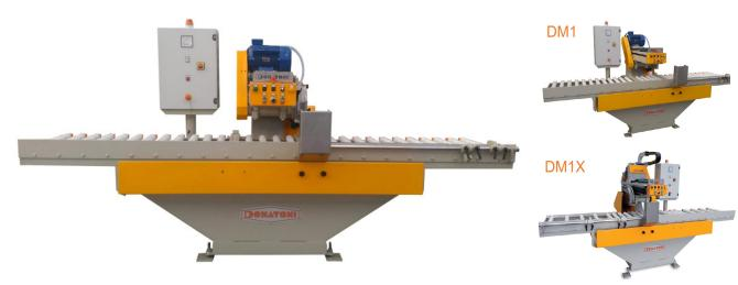
The main feature of the DONATONI cross cutting machine type DM1X is its flexibility in being able to cut both marble and granite, allowing the operator to vary the diameter of the blade autonomously (400 for marble and 350 for granite).
