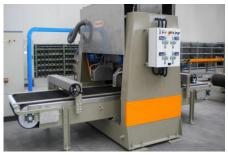
FL linear trimming machines are part of the wide range of trimming machines designed and built by DONATONI for single-pass lengthwise cutting of strips and tiles with the manual positioning system.
