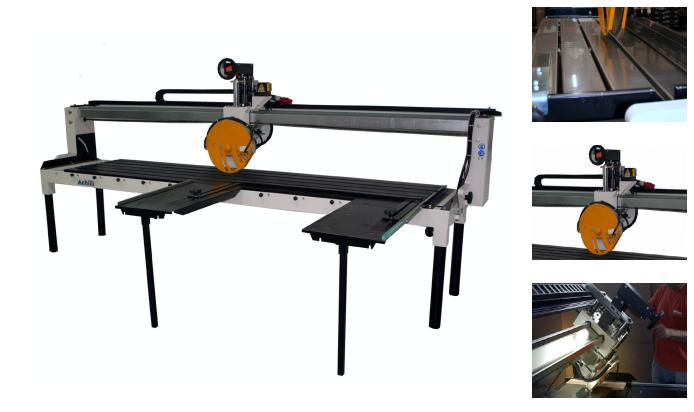
Compact, essential and sturdy saw with fixed bridge and manual head feed for marble and granite slabs; the bridge tilts and the water tank with built-in recycling pump makes it the perfect for small and large stone fabricating shops. It is equipped with 1 or 2 side extension tables to enlarge the working surface and facilitate the positioning of the slabs.
