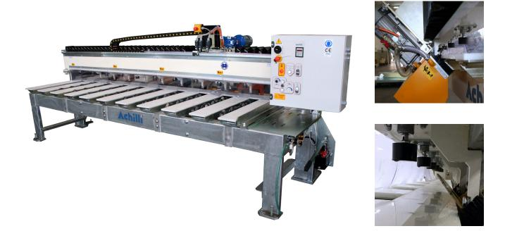
Professional stone saw for tilted cuts designed to work slabs "face down", it allows to perform perfect 45 degree cutting even on uncalibrated slabs. No width limitation of the slab to process; even the most narrow strips can be machined thanks to the special pneumatic pistons blocking the stone. The maximum cutting precision is guaranteed by the head travel on linear guides fitted with recirculating ball slides and by the position of the blade cutting from bottom upwards.
