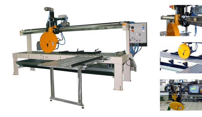
Mono block saw with fixed bridge for stone and sintered material slabs equipped with a compressed, rectified and chromed "active beam" guaranteeing the utmost accuracy. The worktable extensions widen the worktable facilitating the positioning of large slabs and the head feed is motorised with variable speed adjustment in both directions. A special optional device permits to carry out parallel cuts.
